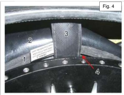
Be cautious with this suggestion! Oil is the enemy of a seated BL Bead. Conservatively lubricate the AC envelope just above the Bead with an oil-dampened Q-Tip. This helps the Bead freely move to its proper position as the beadlock is inflated. Avoid putting oil on the Bead or any other part of the BL or rim.
