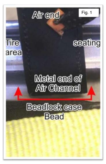
This leads to the Bead struggling to move up and on top of the AC envelope in the direction of the arrows. This tears (uncovers) the leading edge of the envelope and exposes the metal end of the AC. The high-pressure inner tube can now seal off the exposed metal valve stem opening and prevent airing down.
