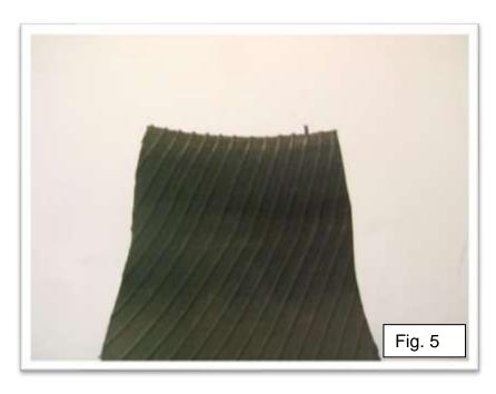
center. Even our heavy-duty, custom-made tubes cannot always survive this. The tire bead must be placed *directly on* rim drop center metal.
