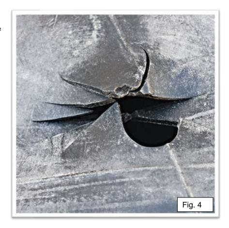
**CAUSE:** The tire bead's sharp, sawtooth edge causes tube failure two ways. One way relates to a weak, stretchy BL case. This was the case for the Australian Stauns that we no longer import. This is fully explained here. — link to "Staun Tread strength" on page <a href="https://www.coyoteents.com/beadlock-tests-and-features/">https://www.coyoteents.com/beadlock-tests-and-features/</a>). This link also explains why the stronger Coyote case does not stretch.
