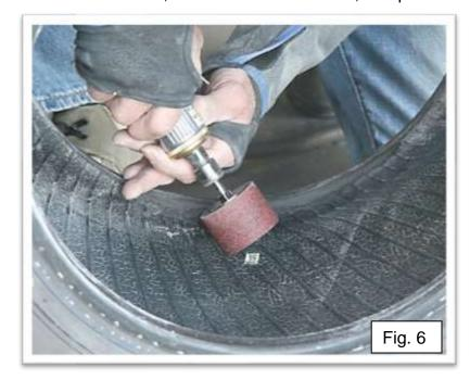
Your goal is to slightly round the tire bead edge as shown. Does this make for leaky tires? I've never experienced or heard of rounding causing tire bead air leaks.
