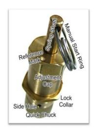
**PARTS:** This Coyote automatic tire deflator outside view shows the four brass parts, the stainless-steel Manual Start Ring and identifies features (Reference Mark, Side Hole and Quick Chuck).
